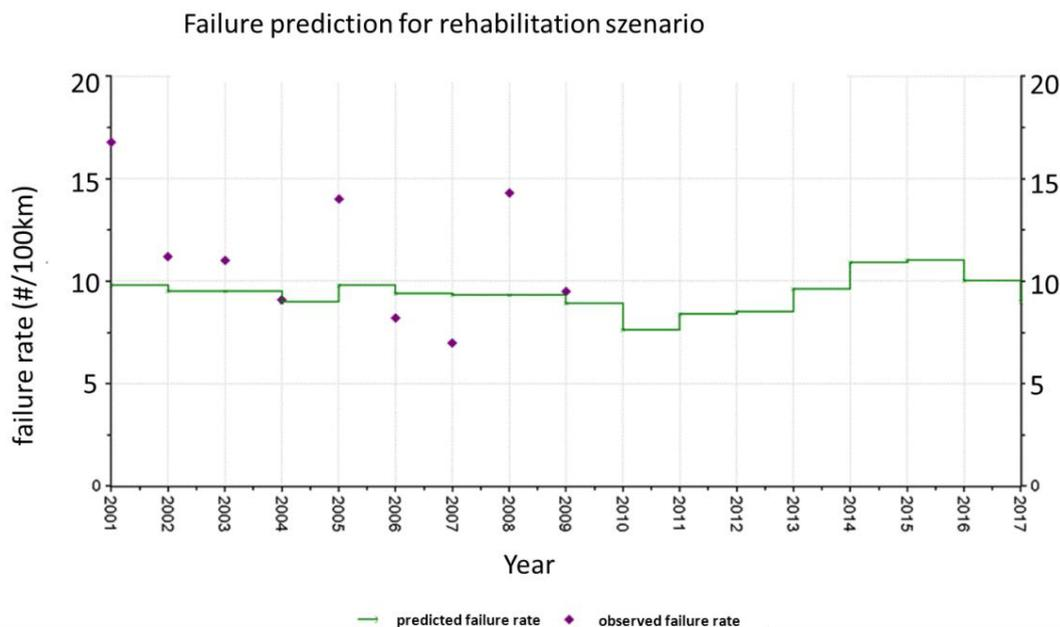
Figure 4: Failure prediction for the chosen rehabilitation scenario of the Viennas Water Supply network (PiReM; 2010)
