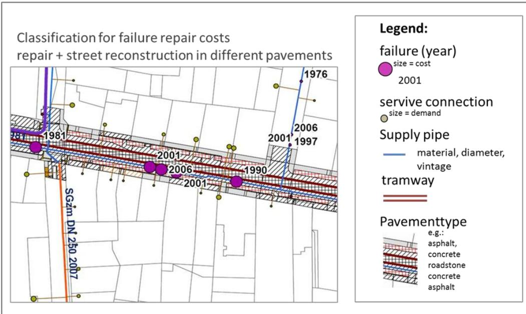
Figure 3: Detailed failure cost specification based on street and pavement type and repair type
